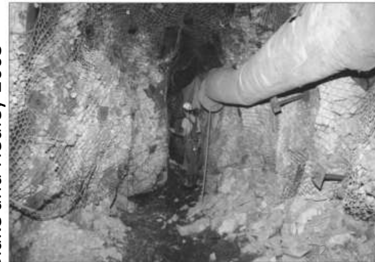
Burst-induced closure within stope
