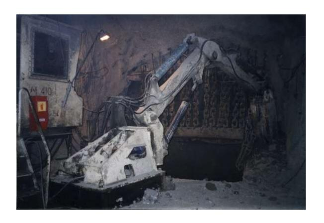
Automated hydraulic breakers exist in underground mines (eg Codelco Andina). Need to provide a mobile platform
